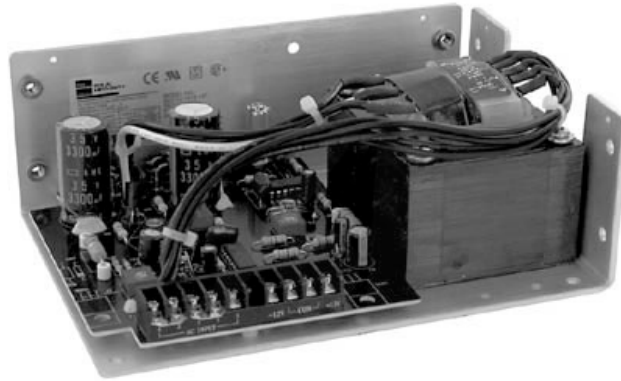
Figure 3.4: Regulated power supply for controller box.
